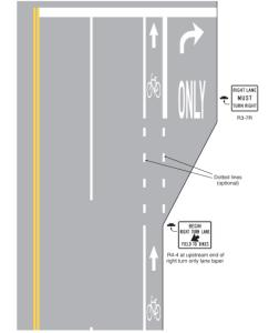
to merge across the right turn lane. One solution to this problem in areas where consistent bicycle traffic is expected is to provide shoulder space between the through travel lanes and the right turn lane. This would be similar to the standard bike lane design shown at right (figure 9C-4 from the California MUTCD), except there would be no bike lane markings included.
